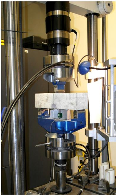
applied load was automatically reduced (unloading phase) when the load passed the maximum value and was about 95% of the peak load. When the applied load was reduced to ca. 100 N, reloading was applied. The cycles of loading and unloading were repeated four times, and then the specimen was loaded up to failure. At the same time, each successive cycle, after the initial, last no longer than 1 minute.
