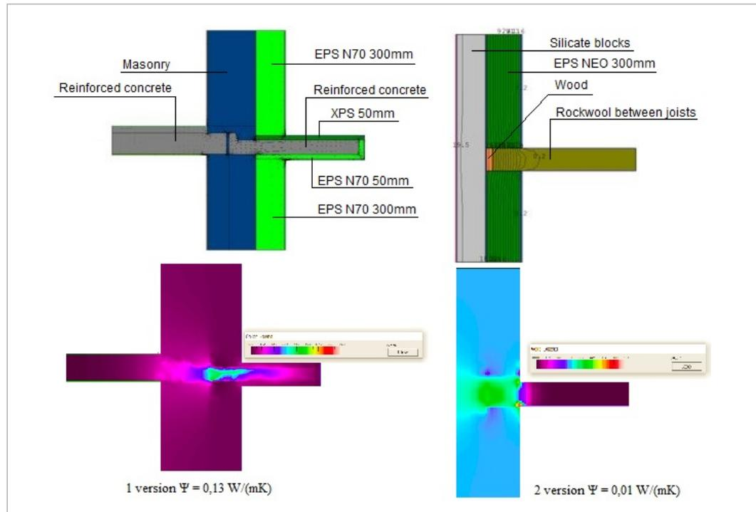
Firstly, building's energy consumption calculations were made including heat losses through first version of linear thermal bridges. As it is shown in table 2, energy consumption of linear thermal bridges consist 8.6 % of total building's energy consumption.
