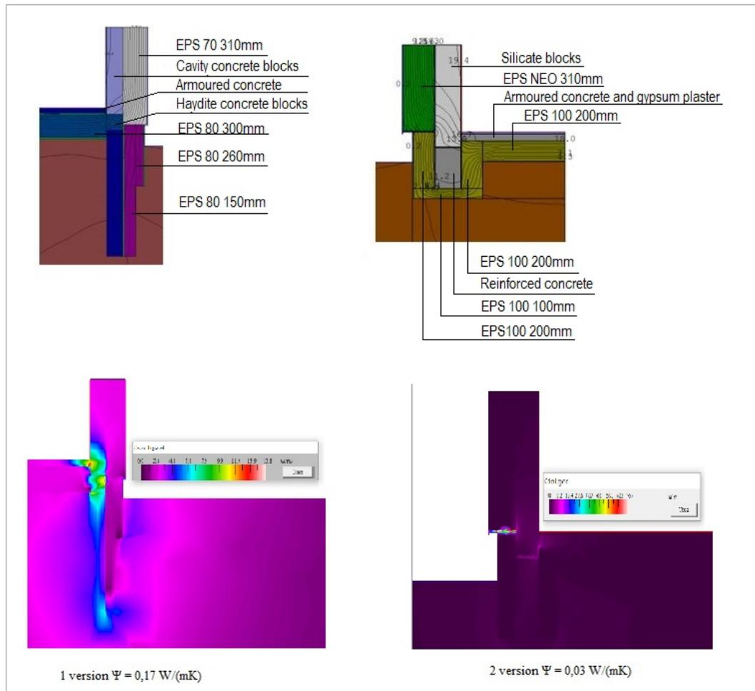
The difference between window position is shown in fig. 9. First example shows window installation directly into lintel, while second example shows window installation in insulating material. Result of heat transfer coefficient is changing more than three times - from 0.10 W/(m·K) to 0.03 W/(m·K).
