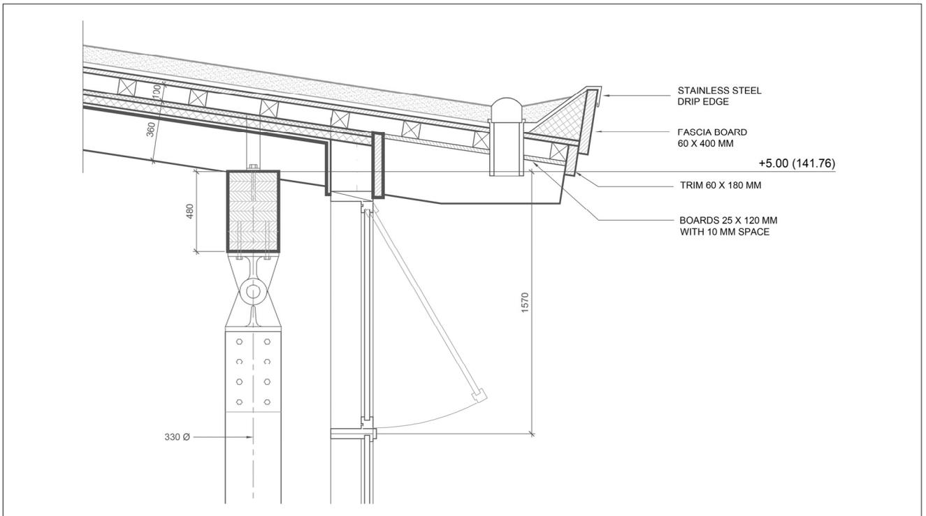
**Fig. 5.** Roof detail
