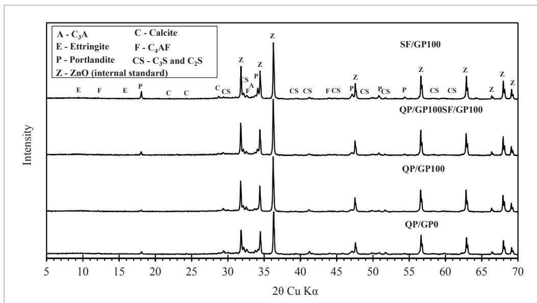
0.2645; 0.2610; 0.2189 nm while  $C_3S$  phases were found at  $d$  equalling 0.3036; 0.2773; 0.2748; 0.2604; 0.2181 nm. Experiment cleared out, that glass powders tends to increase hydration of Portland cement.
