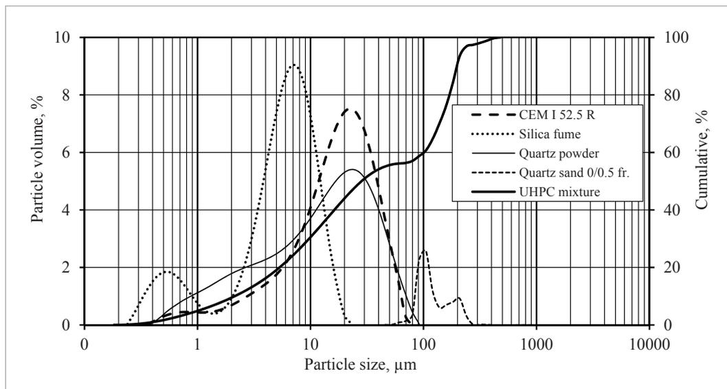
**Quartz powder (QP).** The main properties of quartz powder: the bulk density is  $900 \text{ kg/m}^3$ ; the density -  $2671 \text{ kg/m}^3$ ; the specific surface (by Blaine) -  $3450 \text{ cm}^2/\text{g}$ ; the average particle size -  $18.12 \text{ }\mu\text{m}$ . The particle size distribution is shown in Fig. 1.
