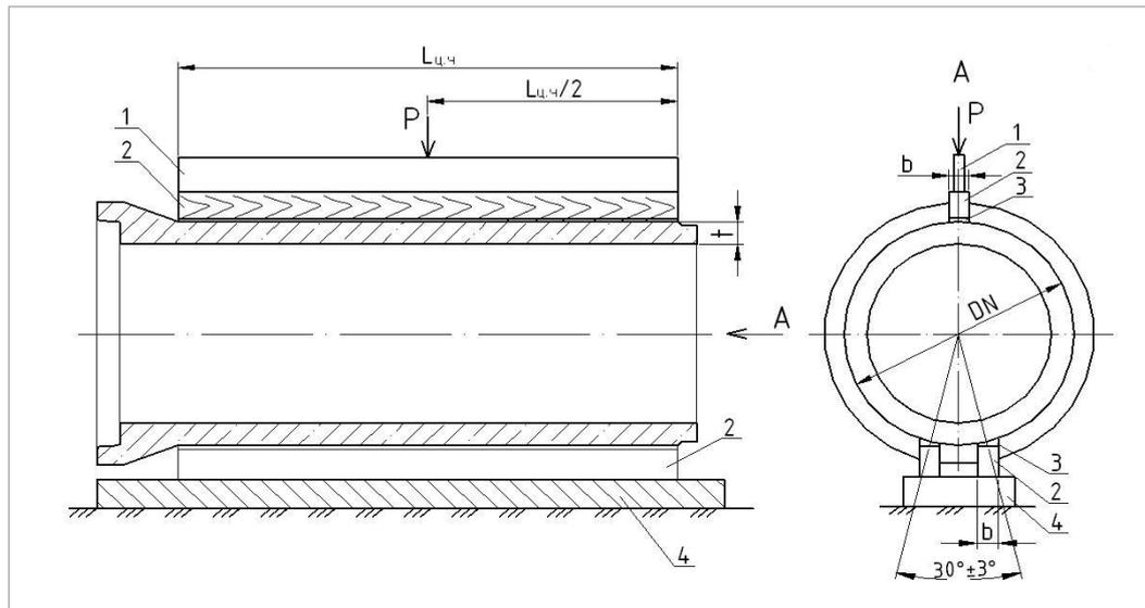
regards the sections located at the level of the horizontal diameter, the lining and its anchoring elements fall into compression zone. If the lining is made of polyethylene with initial elasticity modulus of below 1000 MPa and its anchoring elements are made as solid ribs, strength properties of the sections are reduced significantly.
