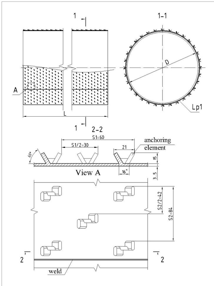
The schemes of inner linings of both types of anchoring elements are presented in Fig. 6 and 7. The load was applied in steps adopted for pipe testing. At each step of loading, concrete elements with tensile deformations exceeding the limit of  $\approx 0.15\text{‰}$  (obtained in an experimental way) were removed and recalculation was performed.
