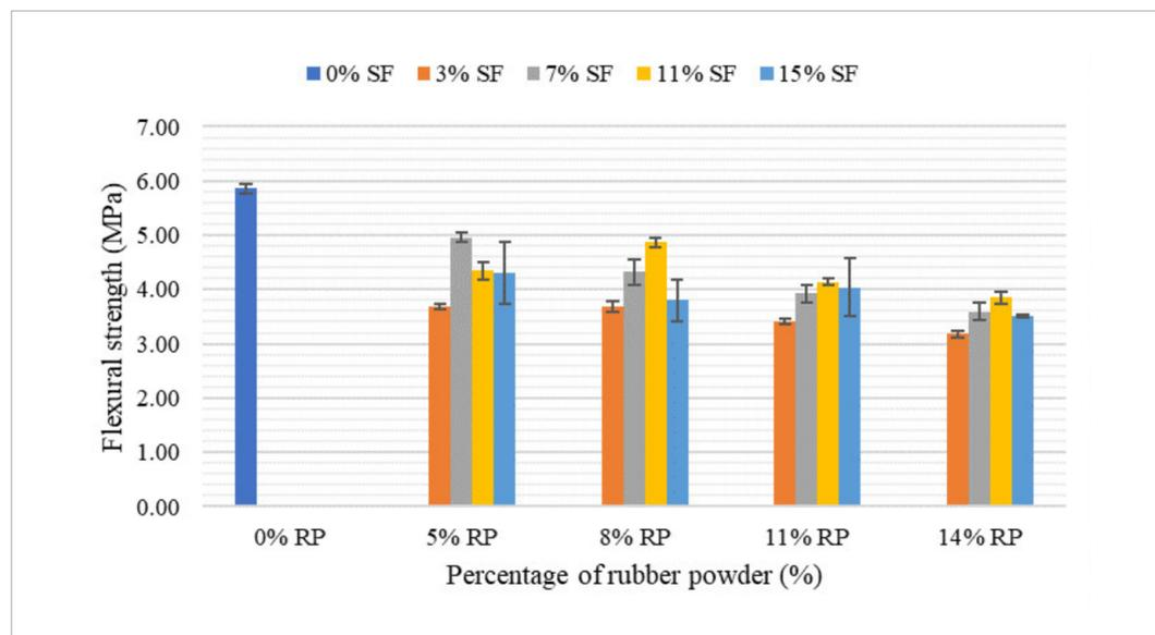
Like the samples for a 21 MPa design, the results of the flexural strength in a 28 MPa concrete, the samples of the experimental concretes did not achieve an increase over the standard concrete which had 5.03 MPa. Fig. 16 shows that the highest strengths are given by 8% rubber powder with 11% silica fume, with a value of 4.67 MPa, followed by 5% rubber powder with 7% silica fume, which was 4.57 MPa, followed by 11% rubber powder with 11% silica fume, giving a value of 4.57 MPa.
