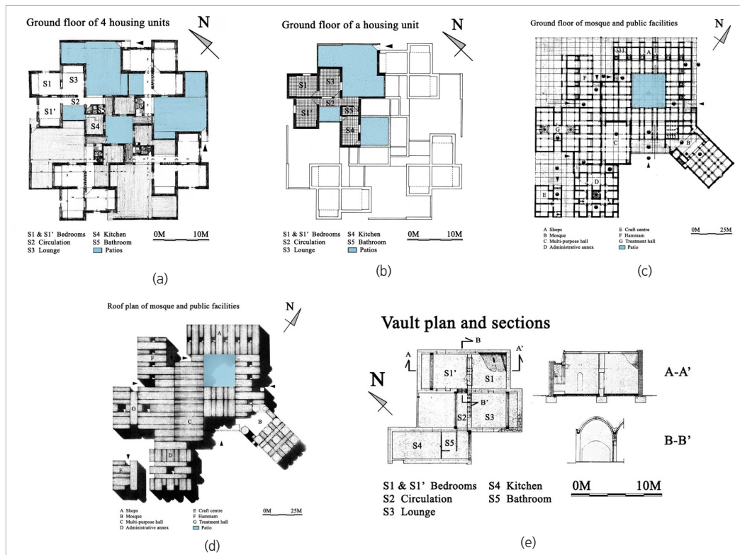
Fig. 14 Plans for Maader Village: (a) ground floor plans of 4 housing units and (b) ground floor plans of 1 housing unit (c) ground floor and roof plans of the mosque and public facilities (d) vault plan and section (e). Source: Authors
