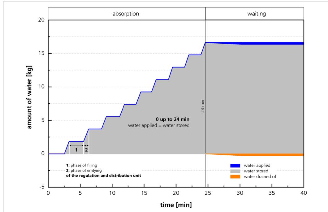
After the water application was stopped, water continued to leak from the module and stopped after a test period of approx. 30 minutes. At the end of the test period, the amount of water absorbed by the retention module was 16.4 kg, corresponding to a relative increase in mass of 193%. Table 2 summarizes the findings in terms of the relative increases in mass for the perlite and vermiculite fillings for each of the retention modules used.
