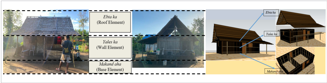
Fig. 4 The main elements of Rumah Malind Aha in Makaling. Source: authors, 2023
