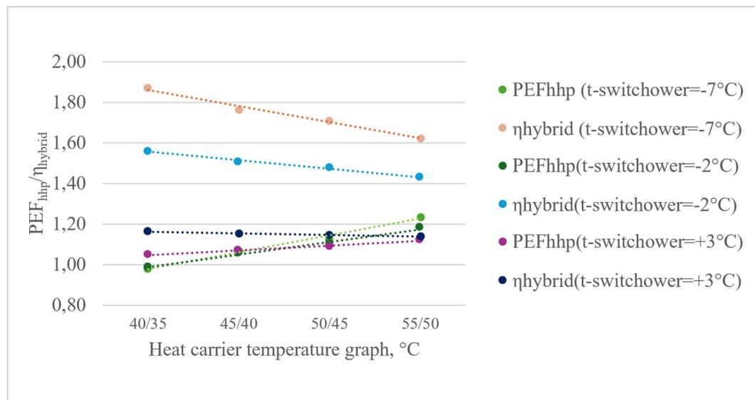
As expected, hybrid heating unit's performance parameters worsen with increased heat carrier temperature graph (total efficiency decreases and primary energy factor increases). It can also be observed that the magnitude of performance parameters change is influenced by switchover temperature setting. When changing the temperature graph from 40/35 to 55/50 °C the changes are as follows:
