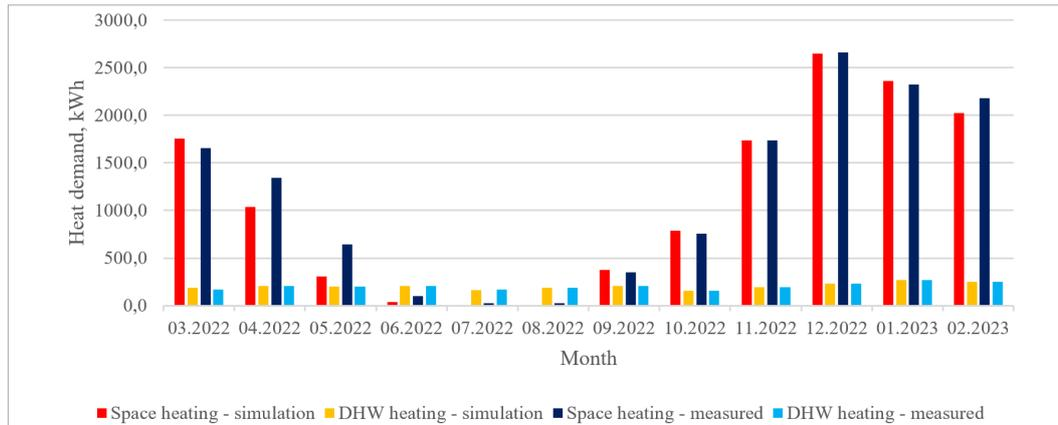
From Figure 4, it can be seen that the simulated space heat demand is very close to the measured. In most months the difference between simulated and actual space heating is no larger than 100 kWh. Months with lowest space heating demand simulation accuracy are:
